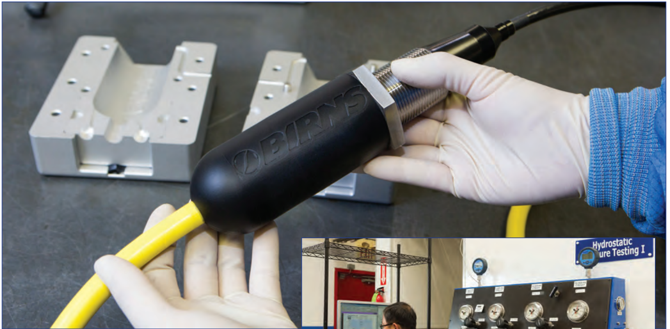
(Top) After the polyurethane overmolding process, a penetrator is removed from its aluminum mold and ready for testing. (Middle) A six-cycle saltwater hydrostatic pressure test is performed, with the outboard side of the penetrator held to pressure of 1,000 psi. (Bottom) Final custom penetrator cable assemblies for the 68-foot Deepstar.
