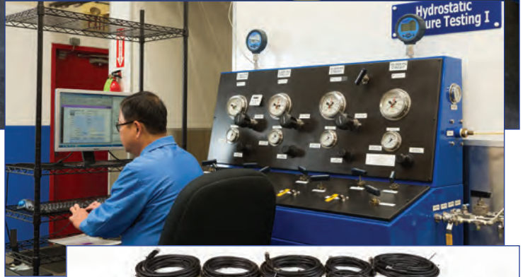
(Top) After the polyurethane overmolding process, a penetrator is removed from its aluminum mold and ready for testing. (Middle) A six-cycle saltwater hydrostatic pressure test is performed, with the outboard side of the penetrator held to pressure of 1,000 psi. (Bottom) Final custom penetrator cable assemblies for the 68-foot Deepstar.
